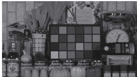
1 lx, 42 dB with built-in PGA + 6 dB in rear end, at F1.4 (black and white model)
