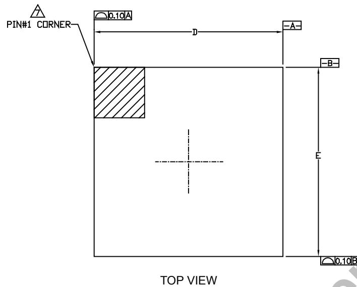
Figure 5-1. Top View of the A12A25 Package.
