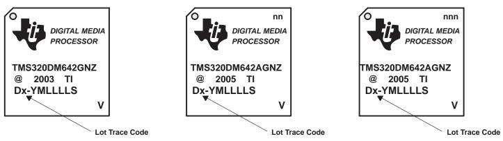
"nn" and "nnn" represent the device speed for the -500, -600 and -720 MHz devices **only** (both commercial and extended temperature).
