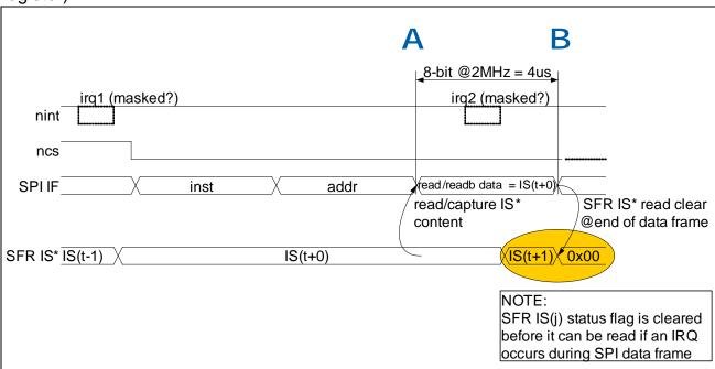
Figure 58 ISx Readout Set Clear Collision
