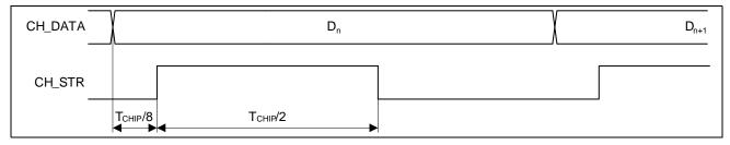
Figure 50 Timing of the Transparent Mode - Chip Data and Strobe
