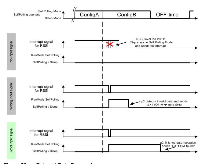
Figure 52 External Data Processing
