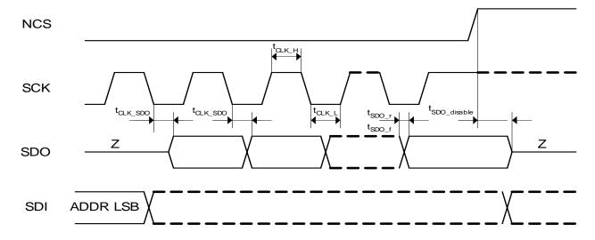
Figure 66 Serial Output Timing
