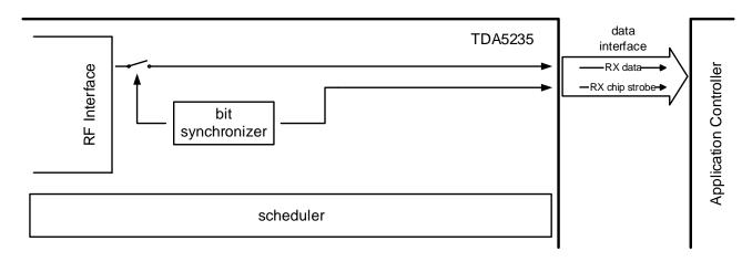
Figure 49 Data interface for the Transparent Mode - Chip Data and Strobe
