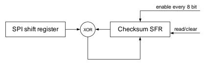
Figure 63 SPI Checksum Generation
