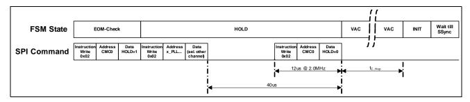
Figure 71 HOLD State Behavior (INITPLLHOLD enabled)
