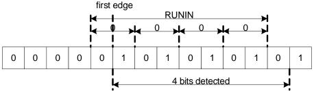
Figure 20 RUNIN Generation Principle
