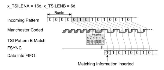
Figure 29 8-Bit Extended TSI Mode
