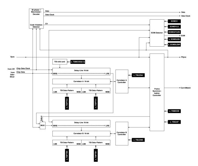
Figure 26 Frame Synchronization Unit
