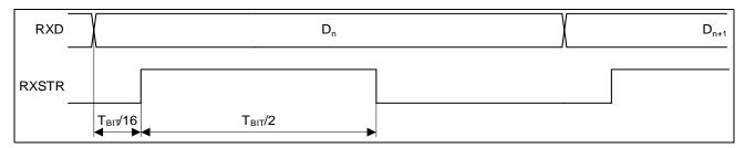
Figure 48 Timing of the Packet Oriented Transparent Payload Mode
