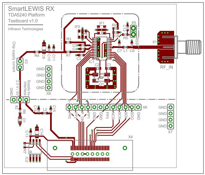
Figure 97 Test Board Layout, Component View
