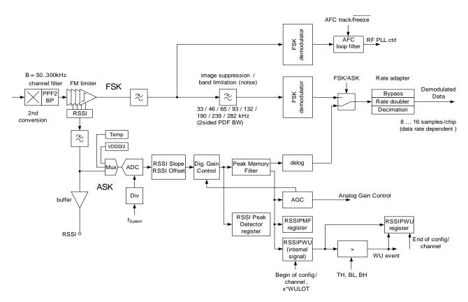
Figure 10 Functional Block Diagram ASK/FSK Demodulator
