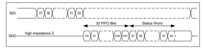
Figure 55 SPI Data FIFO Read
