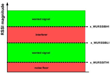
Figure 24 RSSI Blocking Thresholds
