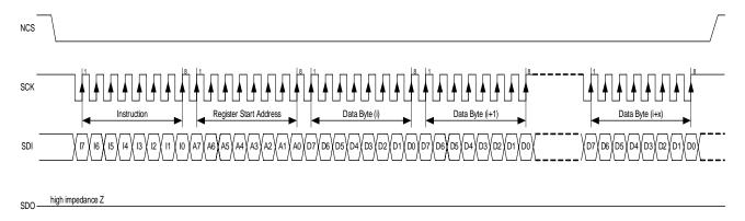
Figure 62 Burst Write Registers
