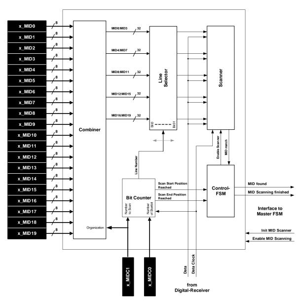
Figure 35 4-Byte Message ID Scanning
