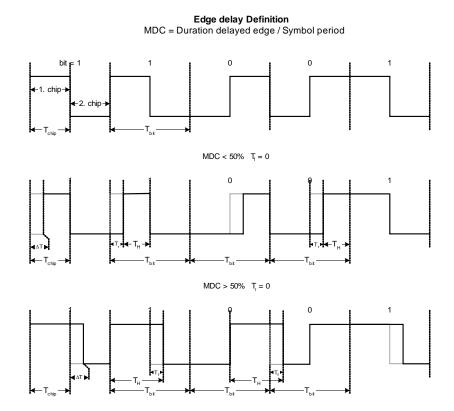
Figure 90 Definition C: Edge delay definition
