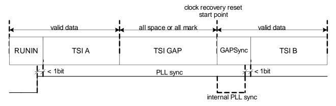
Figure 31 Clock Recovery Gap Resynchronization Mode TSIGRSYN = 1
