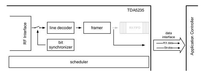
Figure 47 Data interface for the Packet Oriented Transparent Payload Mode
