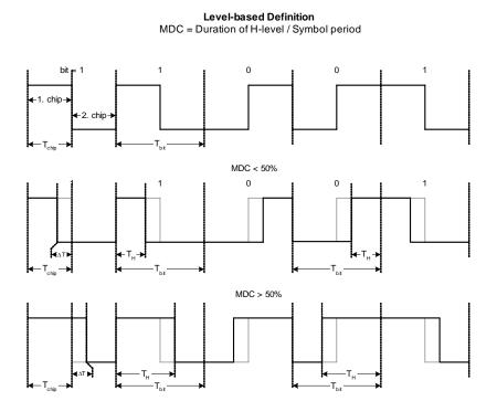
Figure 88 Definition A: Level-based definition
