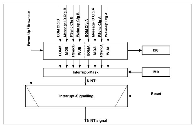
Figure 56 Interrupt Generation Unit
