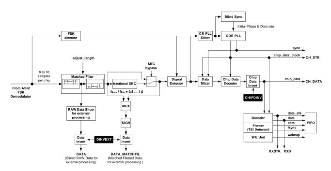
Figure 15 Functional Block Diagram Digital Baseband Receiver
