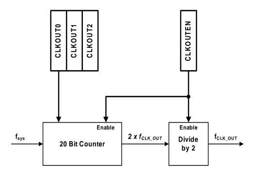
Figure 8 External Clock Generation Unit
