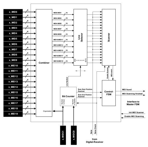
Figure 36 2-Byte Message ID Scanning
