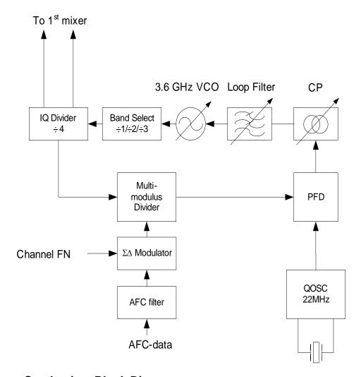
Figure 9 Synthesizer Block Diagram
