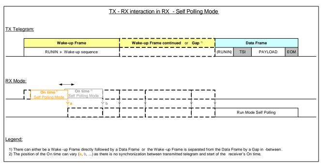
Figure 72 SPM - TX-RX Interaction
