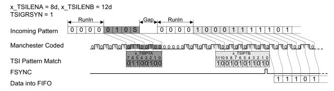
Figure 30 8-Bit Gap TSI Mode
