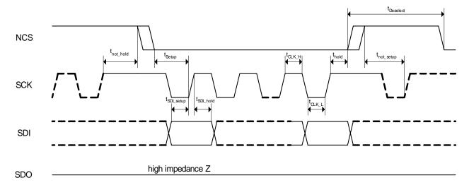
Figure 65 Serial Input Timing
