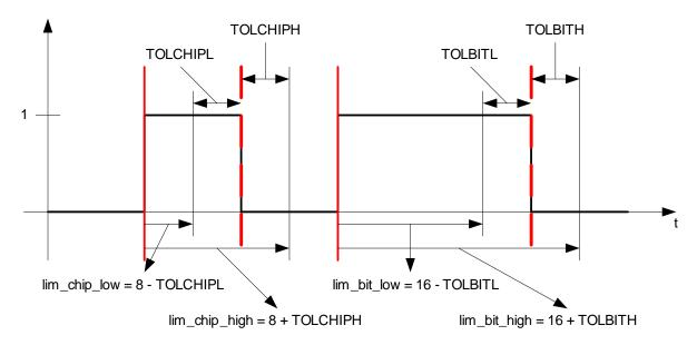
Figure 21 Definition of Tolerance Windows for the CDR
