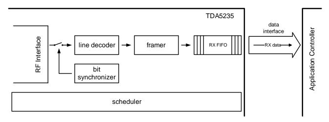
Figure 46 Data interface for the Packet Oriented FIFO Mode
