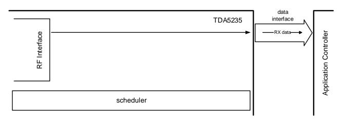
Figure 51 Data interface for the Transparent Modes TMMF / TMRDS
