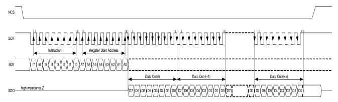
Figure 60 Burst Read Registers
