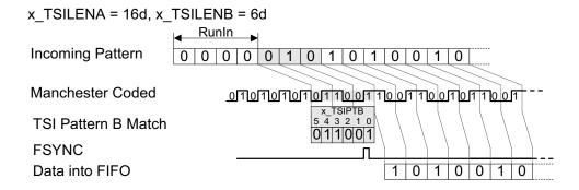
Figure 28 8-Bit Parallel TSI Mode
