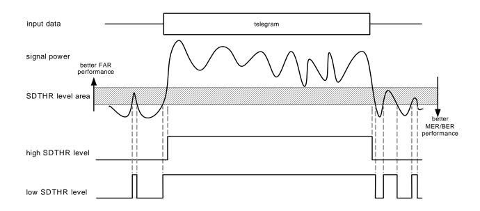
Figure 16 Signal Detector Threshold Level
