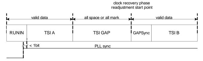
Figure 32 Clock Recovery Gap Resynchronization Mode TSIGRSYN = 0
