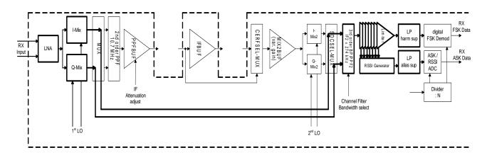
Figure 4 Single Down Conversion (SDC, no external filters required)
