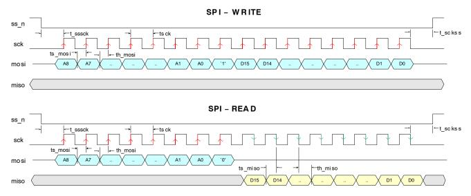
Figure 21. SPI Read and Write Timing Diagram
