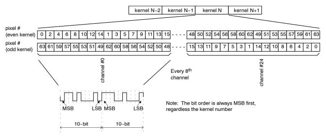
Figure 39. Data Output Order for 4 LVDS Outputs when Subsampling is Disabled
