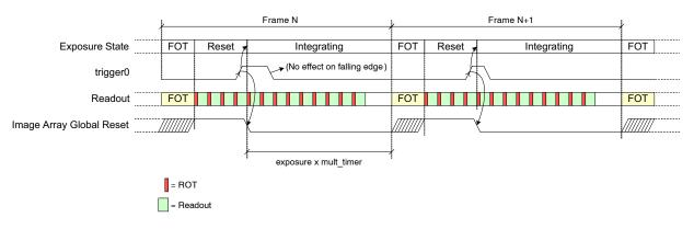
Figure 24. Exposure Time Control in Triggered Global Mode (Master)
