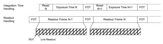
Figure 11. Pipelined Shutter Operation in Master Mode
