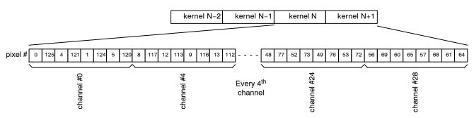
Figure 46. Data Output Order for 8 LVDS Output Channels in Subsampling Mode on a Color Sensor
