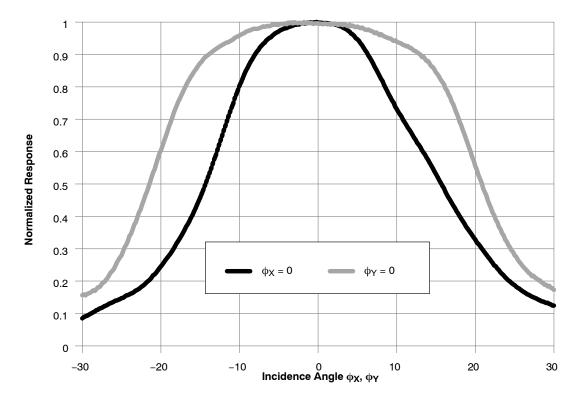
[degrees deviation from normal] Note that the photoresponse peaks near normal incidence for center pixels.
