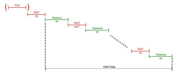
Figure 14. Integration and Readout Sequence of the Sensor Operating in Pipelined Global Shutter Mode with Non-Zero ROT Readout.
