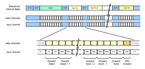
Figure 32. Timeline for Single Window Readout
