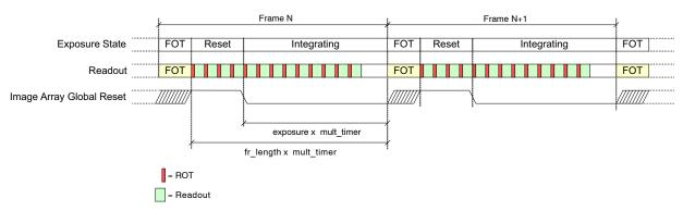
Figure 23. Integration Control for Pipelined Global Shutter Mode (Master, fr mode = 0x1)
