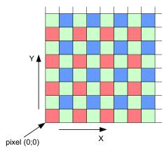
Figure 2. Color Filter Array for the Pixel Array
