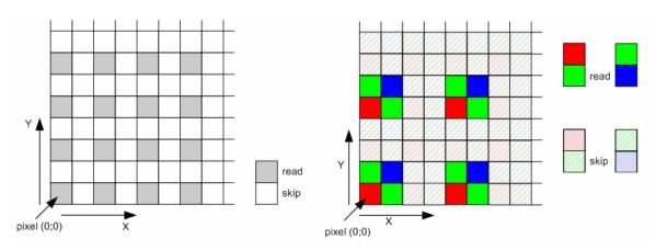
Figure 29. Subsampling Scheme for PYTHON XK
