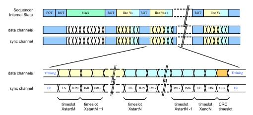
Figure 33. Timeline Showing Readout of Two Overlapping Windows
