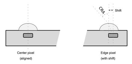
The center axes of the microlens and the photodiode coincide for the center pixels. For the edge pixels, there is a shift between the axis of the microlens and the photodiode causing a peak response incidence angle (CRA) that deviates from the normal of the pixel array.
