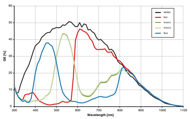
Figure 3. Quantum Efficiency Curve for Mono and Color
