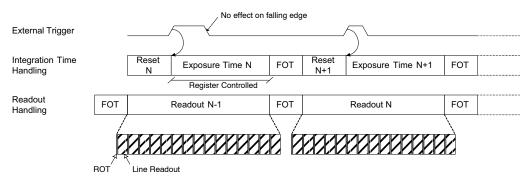
Figure 13. Triggered Shutter Operation in Master Mode
