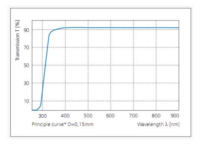
Figure 51. Transmission Characteristics of Glass Lid
