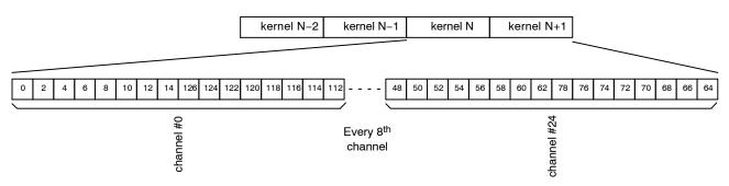
Figure 43. Data Output Order for 4 LVDS Output Channels in Subsampling Mode on a Monochrome Sensor
