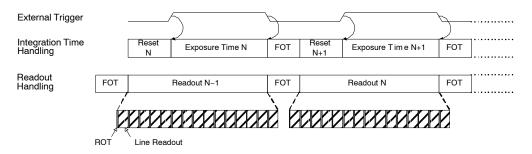
Figure 12. Pipelined Shutter Operation in Slave Mode
