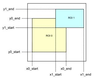
Figure 27. Overlapping Multiple Window Configuration
