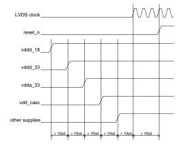
Figure 17. Power-up Procedure
