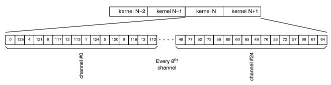
Figure 47. Data Output Order for 4 LVDS Output Channels in Subsampling Mode on a Color Sensor
