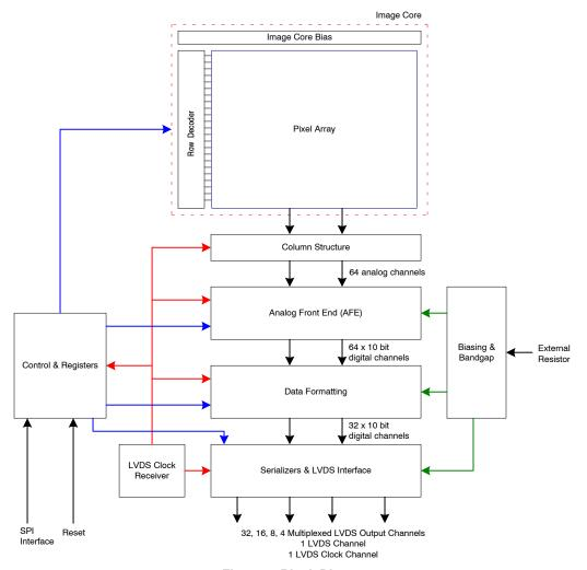
Figure 9. Block Diagram
