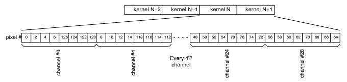
Figure 42. Data Output Order for 8 LVDS Output Channels in Subsampling Mode on a Monochrome Sensor
