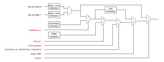
Figure 48. Functional Block Diagrams for the Data Channels
