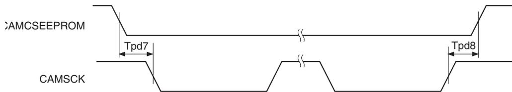
(within the recommended operating range, CAMSCK load capacitance = 29 pF, CAMCSEEPROM load capacitance = 15.5 pF)
