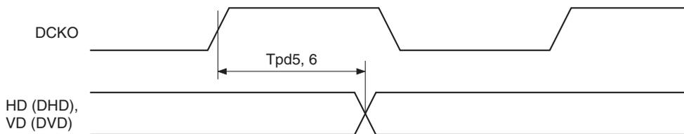
(within the recommended operating range, TGHD, TGVD load capacitance = 15.5 pF)
