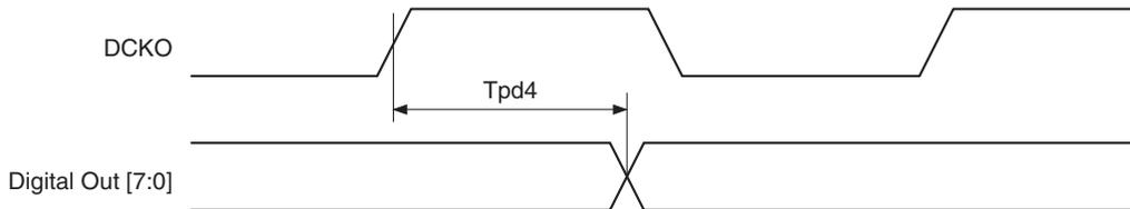
(within the recommended operating range, DCKO, PB[7:0] load capacitance = 15.5 pF)
