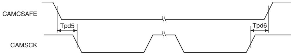
(within the recommended operating range, CAMSCK load capacitance = 29 pF, CAMCSAFE load capacitance = 15.5 pF)
